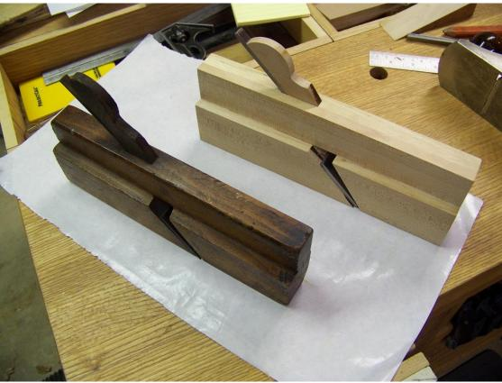
Shown in the next photo is the pair of planes. I have taken the liberty of detailing (the nicks, bevels and rounding the hand hold end) the hollow plane without the benefit of photos.
