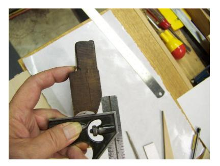
I marked a line on the side, down the length,  $\frac{3}{4}$ " from the sole. A second line was marked on the sole, about  $\frac{1}{16}$ " for the blade(next photo).
