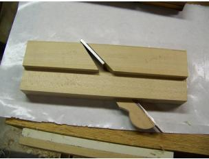
I darkened the blade steel with a black marker, and scribed the profile onto the forward part of the steel (next photo).
