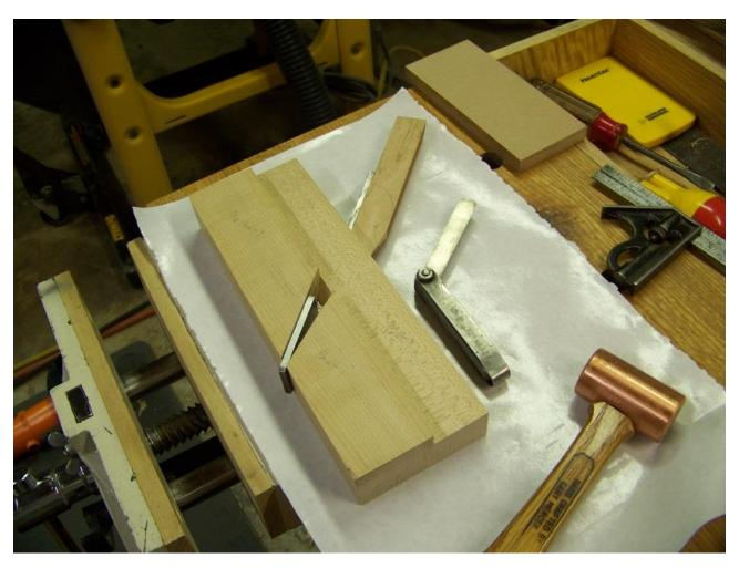
I used a fret saw and a file to shape the upper section of the wedge. The lower part of the wedge will be shaped later (next photo).
