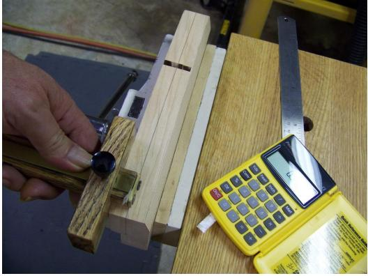
I marked the inside edge of the blade line onto each end of the plane, using my marking gauge. I used a compass to mark the 1" radius, and then extended those lines down the length on each side (next 2 photos).
