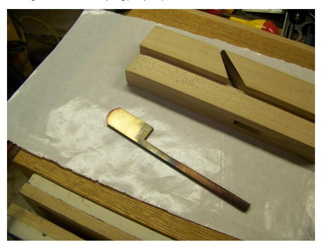
The end of the wedge on the antique ends at about  $\frac{1}{2}$ " from the sole when it is seated and ready to use, and it worked so well, I decided to copy it's features.
