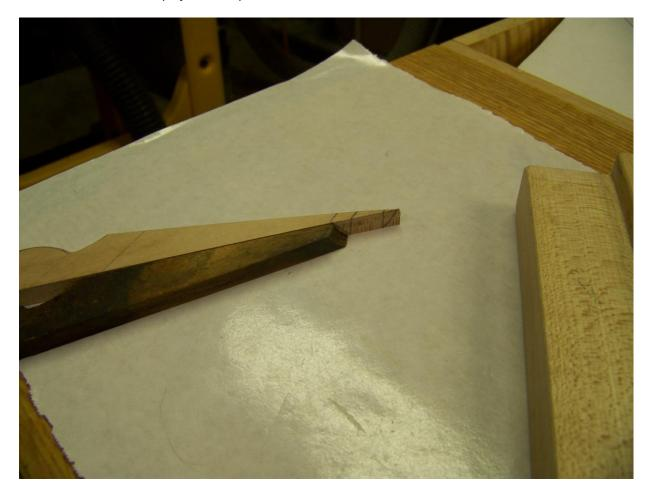
I cut almost to the line, then made a radius with a file.
