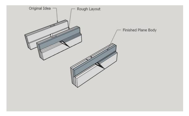
I decided to use a bed angle 45 degrees and a 10 degree wedge. I know tradition is 55 degree bed and a 12–1/2 degree wedge but I already had a wedge jig for making 10 degree wedges, so there it is!
