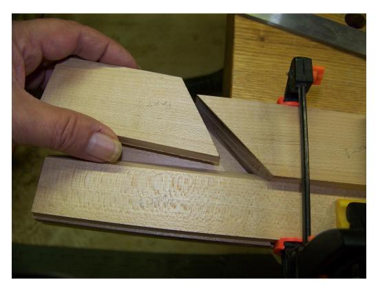
Use the blade steel and wedge to make sure the wedge and bevel edge (on part 3) is a match when the wedge is snug.
