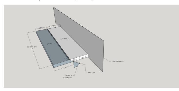
It's time to cut out the wedge pockets. I use a miter saw that I normally use just for 90 and 45 degree angles. I first cut the 45 degree angles on each of the Parts 1, 2 & 4.
