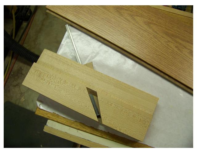
Using a piece of leftover snaplock flooring, I clamped it along with the plane into the vise, so I could use it as a fence to hollow out the sole of the plane (next 2 photos).
