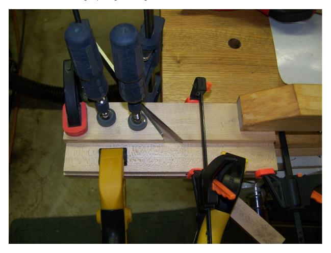
While the glue is drying, you can prepare the long beveled strip (Part 3) for the next step by marking pencil lines where the wedge will be. The pencil lines are marked on the wedge side (wide side) of the part so when you apply glue to the part 3 you can avoid the wedge area. Glue in the wedge area would be difficult to remove.
