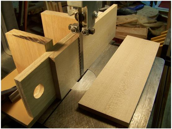
Part 2 and Part 3 are separated from one board before cutting out the wedge pocket. (Print this page to make it easier to follow along)
