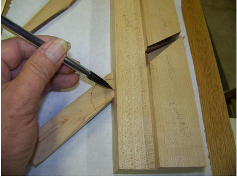
I marked a center point for the arc (next photo) about 1/8" from the upper layout line and drew the large arc, then drew the smaller arc by hand.
