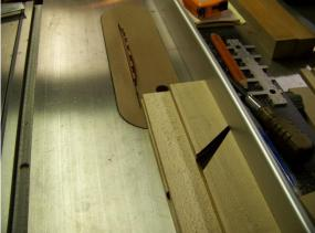
I Begin laying out the wedge using 2 lines marked onto the wedge (next 2 photos). The first layout line is with the blade steel inserted from the bottom (because it has not been shaped yet) with the wedge inserted, then the second layout line is without the blade steel.
