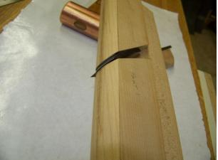
To soften the edges, I marked a  $\frac{1}{2}$ " radius on the rear of the plane (the same as the antique) and shaped it to that line (next photo).
