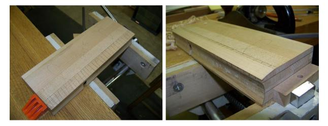
In the photo below you can see that there is about 3/32" of sole on each side of the blade steel (the blade steel is shown with the wedge protruding). I have not shaped the blade or the wedge yet.
