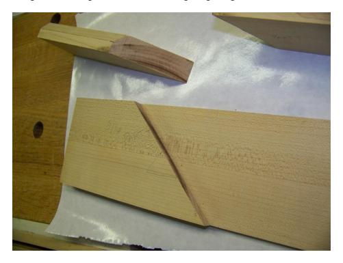
Next I made a temporary wedge (shown below) that was thicker, and square, to check the fit of the parts before gluing any more parts.
