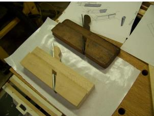
Laying out the sole began by measuring the relief angle on the antique. It measured ¾" upward from the the bottom of the sole (next photo).
