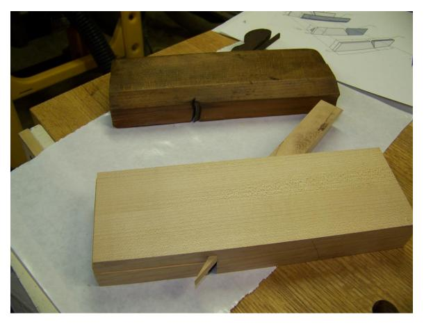
It took about six strokes with my bailey #4 smoothing plane to clean up the sole and make it square with the solid side (not the wedge side). I then used my table saw (solid side face down) to make the top parallel with the bottom (next 2 photos).
