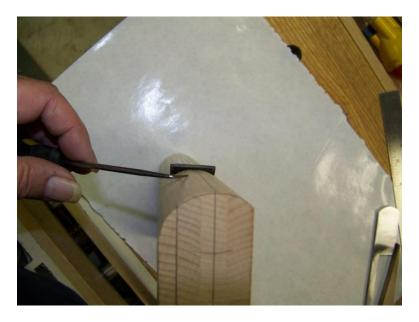
I used a bench grinder to grind the profile at a 25 degree relief bevel.
