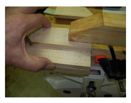
Remember; No glue yet! Part 3 is being used for alignment at this point!
