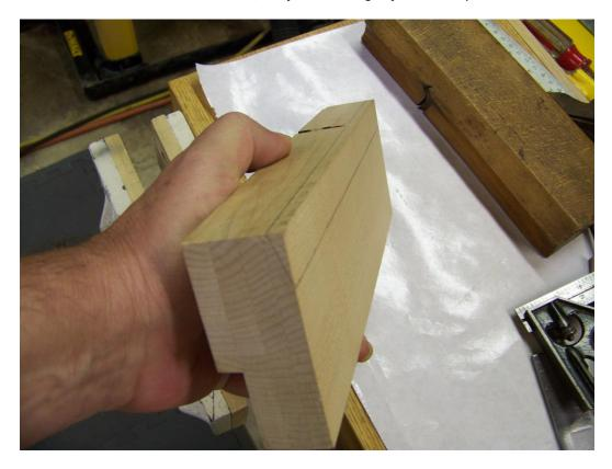
I used my smoothing plane to create the relief bevel. I marked cross lines to see my progress, as I planed down to the lines (next 2 photos).
