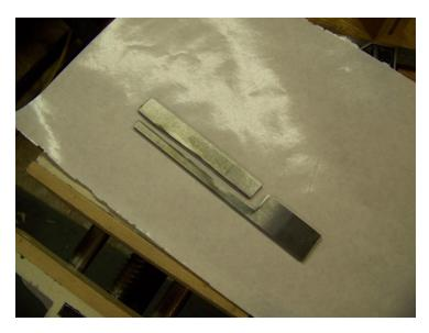
After removing the burrs, I checked the fit (next photo). I am very happy with the clearence (.011") for the mouth opening. The antique has about 1/8". I wanted it to be a tight fit because I have yet to shape the bottom, and I know the clearence will open up as I do that.
