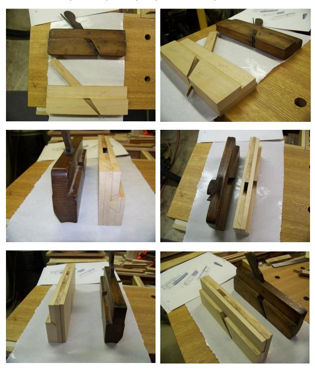
In this photo, note that the combined Parts 2&3 protrude slightly beyond the base line. That is because it is more important to have had it lined up with the long beveled strip, and the wedge pocket when it was glued. A couple of strokes with a smoothing plane will take care of the sole..
