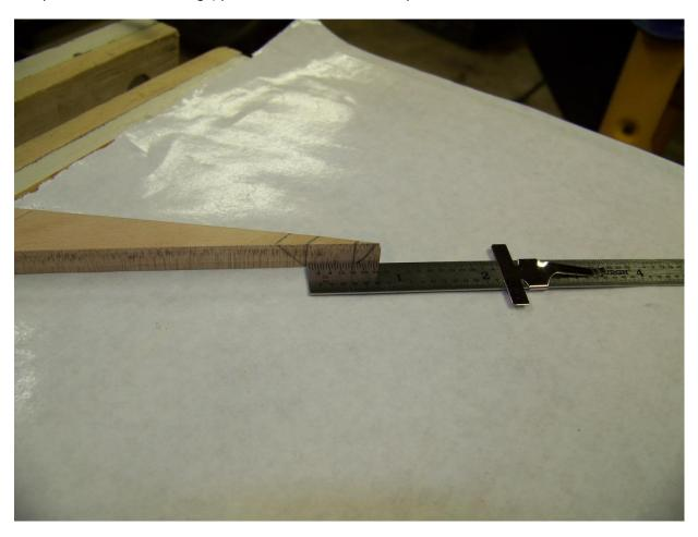
For Clarity, I layed the wedge on the plane body to show the lines marked parallel with the sole. You can clearly only see in this photo the second, third and fourth lines.
