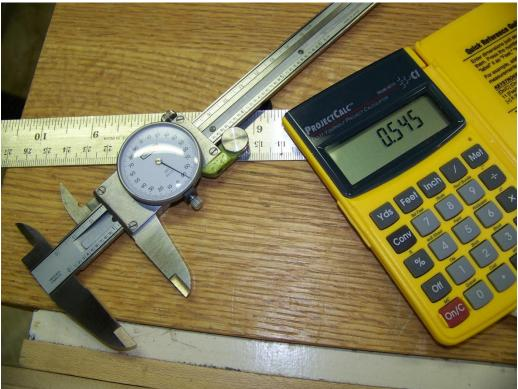
I used the calipers to prick into the wood, so I could set my marking gauge directly, then marked the centerline for the blade. I also marked the centerline onto each end (next 2 photos).
