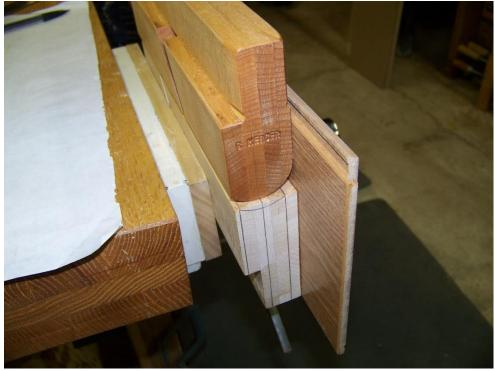
After I had hollowed a bit, I removed the fence and planed up to the layout lines by tilting as I went, checking each end as I went along. The last few stokes are done vertically to define the sole.
