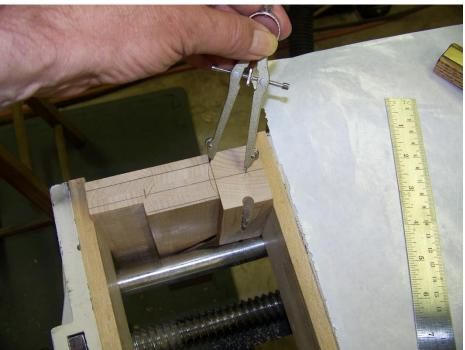
I put the plane into a state of tension, as if the plane was ready to use by using a piece of keystock, and a test wedge(next photo) that was driven into the wedge opening. I just thought that when I shape the sole, it would come out straighter if it had tension.
