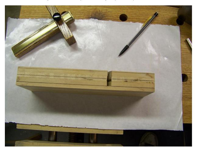
In order to mark the radius onto the ends of the plane, I used a scrap block of wood with a line marked at a right angle. I then clamped the block with the plane(next 2 photos) into the vise to layout the radius. With the compass set to the width of the plane Blade I crossed two lines onto the scrap wood, and then marked the radius line onto each end of the plane.
